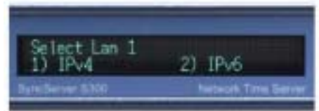
Crisp and bright vacuum fluorescent display offers high readability both near and far. Characters can be large, medium or small. Intensity is user adjustable.
