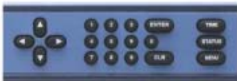
The full numeric keypad is the most efficient way to navigate a menu driven interface. The [TIME] & [STATUS] buttons quickly display the most critical information.
